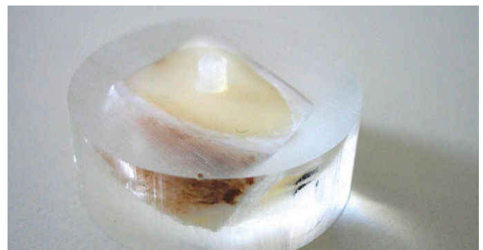
Fig. 4: Specimen for shear bond strength testing according to ISO 29022:2013 (bovine dentin)
